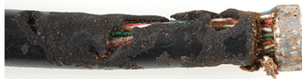
Fig. 4. Example of a 'destroyed' cable sample, i.e. penetrated, by Coptotermes acinaciformis at the Darwin site from the trial with the accelerated container method. Note that the sample has not only been penetrated but large amounts of the polyethylene have been removed as well.
